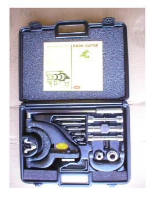
This is the most popular size of the Radii-Cutter line. Designed for 11 inch swing and larger lathes, the 4 inch Radii-Cutters can turn a maximum 4 inch diameter ball. Sockets of 4 inches diameter can be turned to radius depth, and by reversing the "C" yoke, shallow sockets of up to 12 inches in diameter can be turned. Center height of the Models 4S and 4D is 1 5/8 to 1 ¾ inches, and the tool can be shimmed to fit larger machines.
